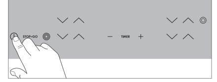
After switching off a single cooking zone or the entire cooking surface, the existing residual warmth will be displayed in the digital displays of the corresponding cooking zones in the form of  $\mathbb{H}$  (for "hot").
